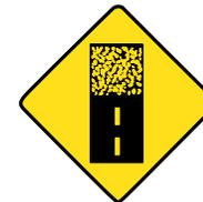
The hard-surfaced pavement changes to an earth road or low-type surface. Slow down.
