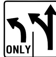
This sign indicates that two lanes of traffic are permitted to turn left. The traffic in the left lane must turn left, traffic in the other lane has a choice.
