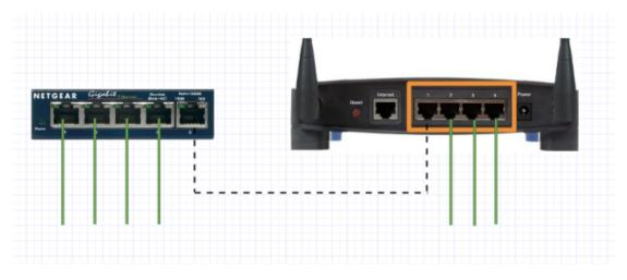
If you need to expand again, it's best to use one of the original ports on the router – while daisy chaining switches together is possible, you will introduce a small amount of latency each time. If there's no other option though because the router is too far, daisy chaining one or two times is still preferable to other technologies like Wi-Fi or powerline.
