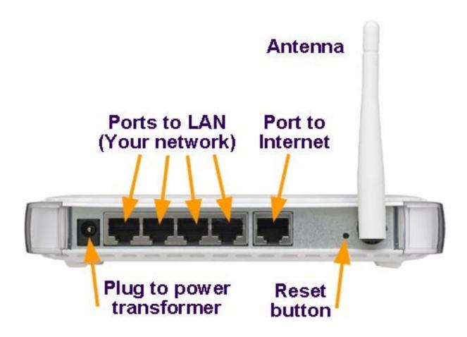
The image above was taken from Netgear's support page, showing the ports on the back of a typical router. Although the WAN port is physically identical to the local network ports, the router will have a built-in firewall for traffic entering that port only – while the internal network is trusted fully.
