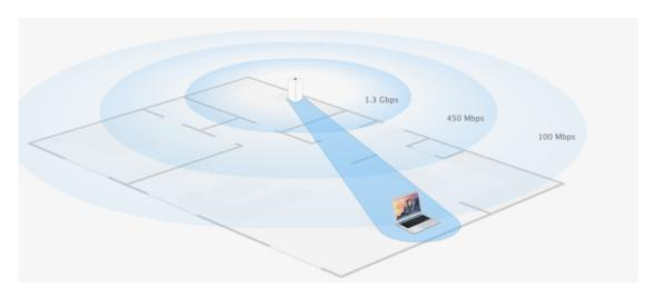
The image above was taken from Apple.com explaining the AirPort Extreme with 802.11ac "beamforming" technology.
