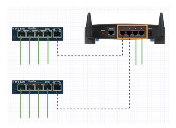
*Do I need crossover cable?* **No**. You may have heard that crossover network cables are used to connect thing like switches and routers, but modern hardware is clever enough to do this crossover in firmware – there is no need to use special cabling. On some switches, you may still have a designated "uplink" port, or even a physical button to change modes – use this as the interconnecting port.
