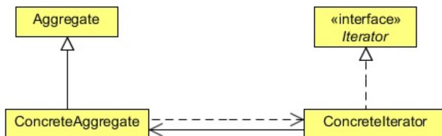
Figure 23.1: - Class diagram
