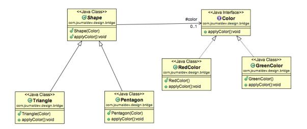
Notice the bridge between *Shape* and *Color* interfaces and use of composition in implementing the bridge pattern.
