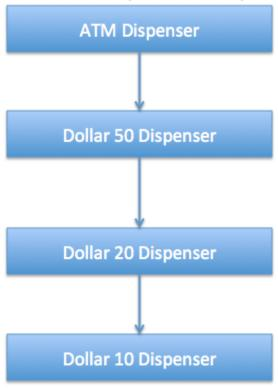
Note that we can implement this solution easily in a single program itself but then the complexity will increase and the solution will be tightly coupled. So we will create a chain of dispense systems to dispense bills of 50\$, 20\$ and 10\$.
