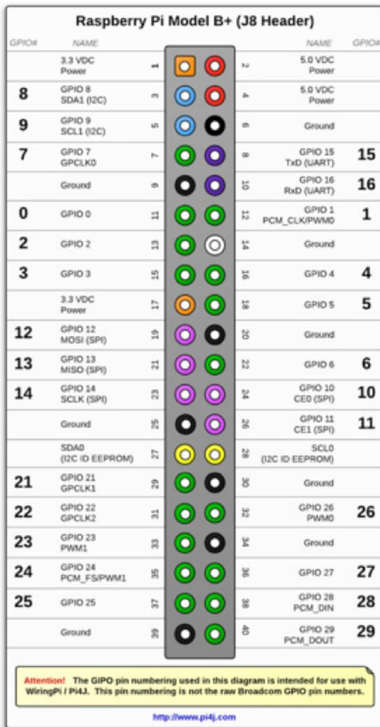
FIGURE 7: PIN ASSIGNMENTS FOR THE PI4J LIBRARY (DIAGRAM BY ROBERT SAVAGE; SOURCE: PI4J.COM/PINS/MODEL-B-PLUS.HTML.)
