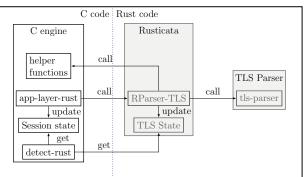
Figure 2. Function calls between C and Rust.
