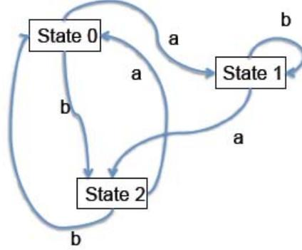
Figure 3.1: A finite state machine with alphabet  $\Sigma = \{a, b\}$  and state set  $S = \{\text{State 0}, \text{State 1}, \text{State 2}\}$ . If pressed, we will make State 0 the initial state and  $\{\text{State 2}\}$  the set of final states.
